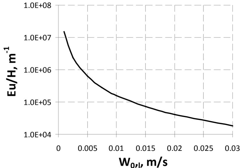
Fig. 1. Dependence of the value of the Euler number on the velocity of the liquid phase.
