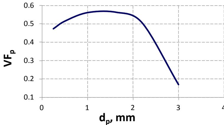
Fig. 2. The effect of the particle size of the catalyst on the volume fraction of the catalyst  $VF_p$ , averaged over the volume of the ebullated bed.
