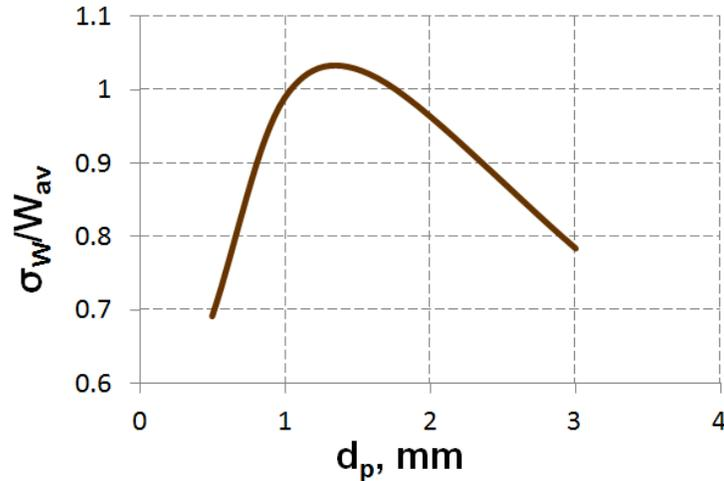
Fig. 3. The effect of the particle size of the catalyst on the liquid velocity inhomogeneity  $\sigma_w$ .
