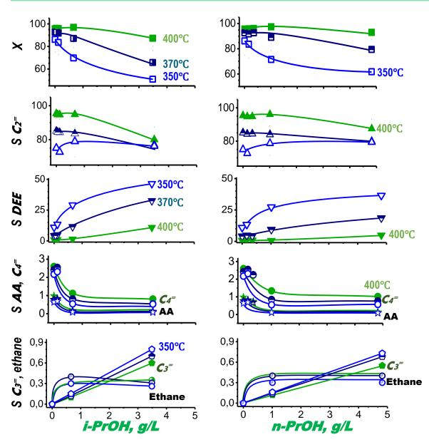
The effect of  $C_3$ -alcohols on ethanol conversion (X) and products selectivity (S, mol%) in bioethanol dehydration at 350, 370 and 400°C
