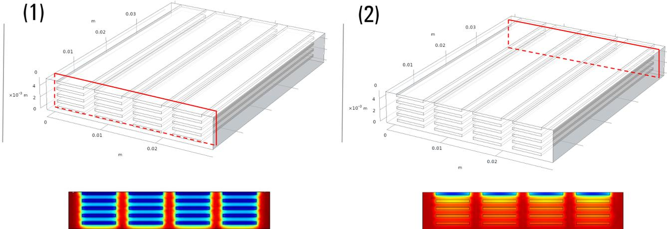
Conversion in different cross-sections of the reactor
