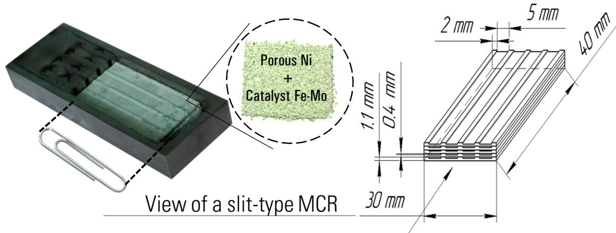
The slit-type MCR consists of 5 porous nickel plates 40 mm long, 30 mm wide and 1.1 mm high. Each plate contains 4 channels 0.4 mm high and 5 mm wide. Finely dispersed particles of industrial Fe-Mo catalyst are evenly distributed within the porous matrix. The channel spacing is 2 mm.
