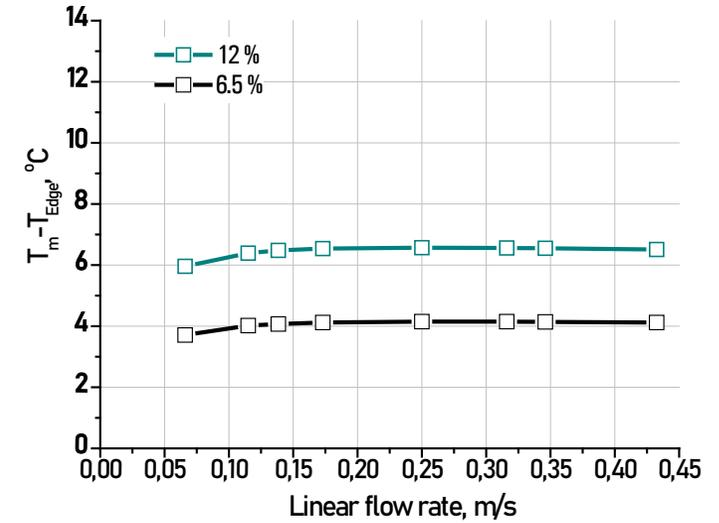
An increase in the edge temperature and methanol concentration is accompanied by the increase in reaction rate and the heat released. This leads to an increase in the temperature gradient relative to the edge temperature both at the outlet from the central channel and at the hot spot (Slide 8).
