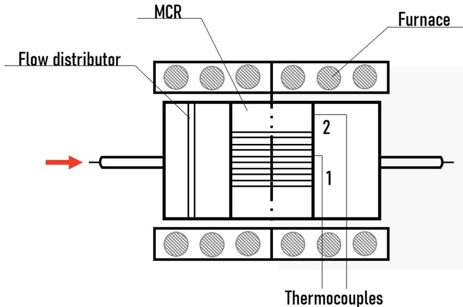
The reactor is positioned inside the furnace. Feeding device ensure perfect mixing at the inlet of the channels. Porous membrane ensures uniform flow distribution.
