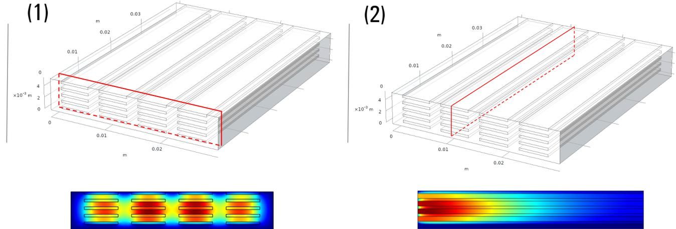
Temperature distribution in different cross-sections of MCR
