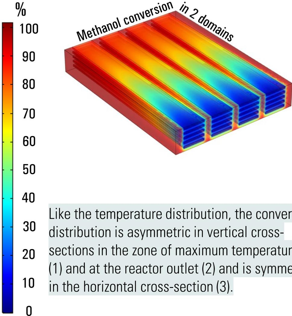
Like the temperature distribution, the conversion distribution is asymmetric in vertical cross-sections in the zone of maximum temperatures (1) and at the reactor outlet (2) and is symmetric in the horizontal cross-section (3).
