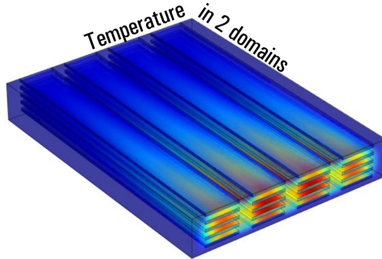
The temperature distribution in cross-sections (1) and (2) is asymmetric due to the fact that the upper row of channels is bounded by the reactor wall and the lower one by the catalyst plate. In cross-section (3), the temperature distribution is symmetric.
