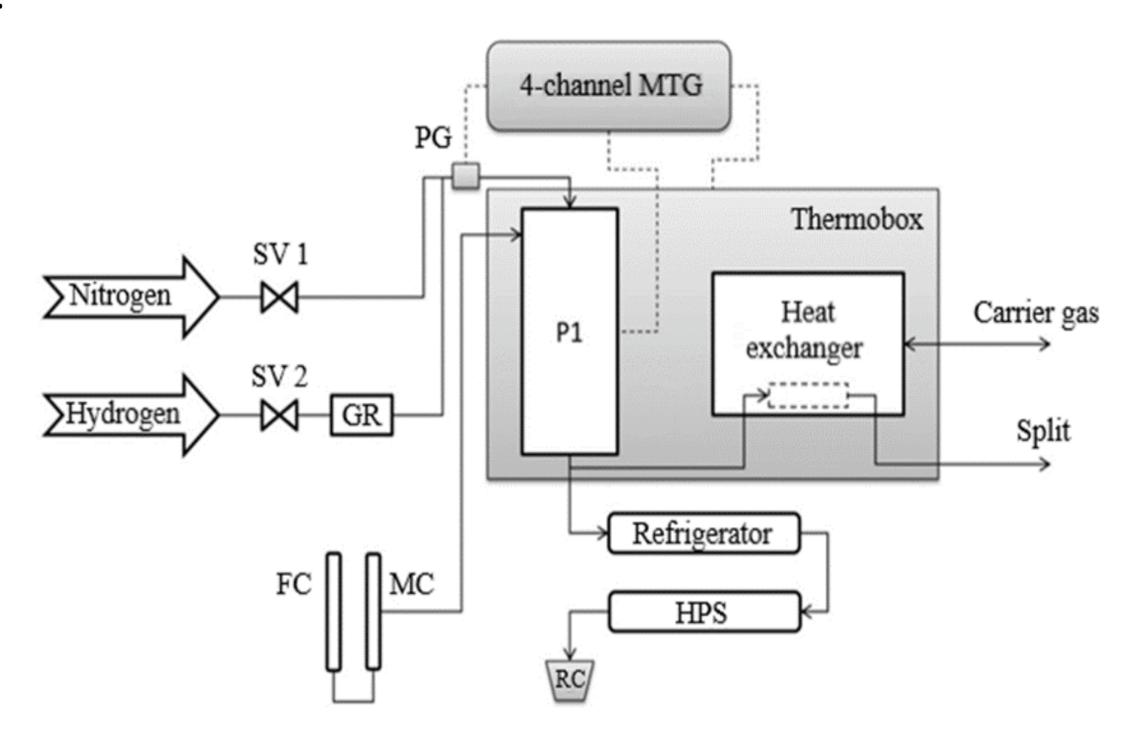
Fig. 2. Technological diagram of a laboratory catalytic installation
