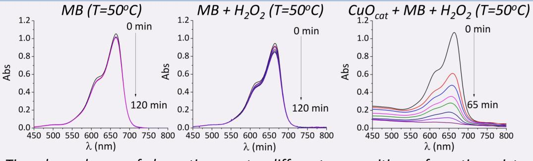
Time dependences of absorption spectra different compositions of reaction mixture
