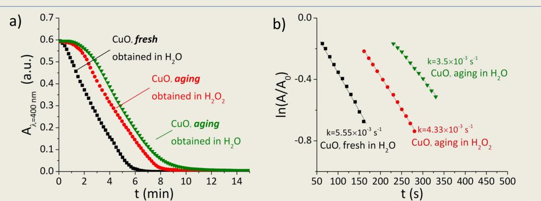
Kinetic dependences of NP consumption (a) and  $\ln(A/A_0)$ -time plots (b) for samples obtained in  $H_2O$  and  $H_2O_2$
