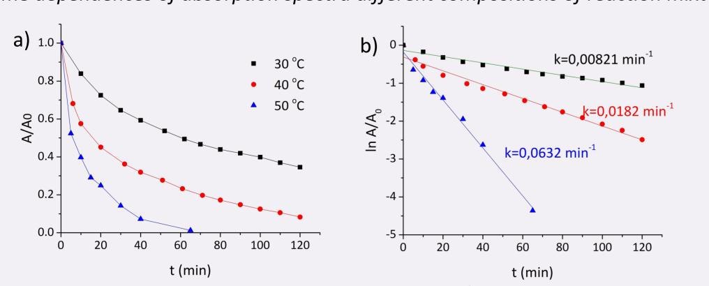
Kinetic dependences of MB consumption (a) and  $\ln(A/A_0)$ -time plots (b) at deferens reaction temperature
