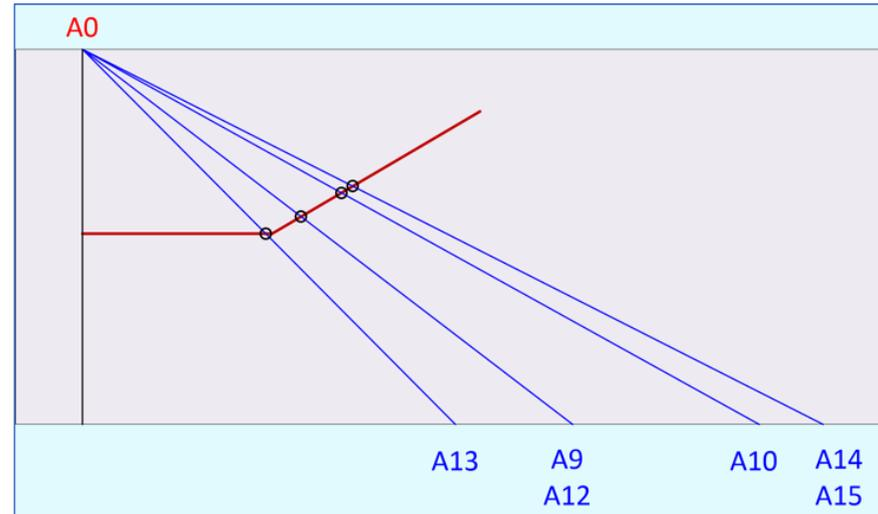
Sketch of the fracture (red line) and ultrasonic wave rays (blue lines).
