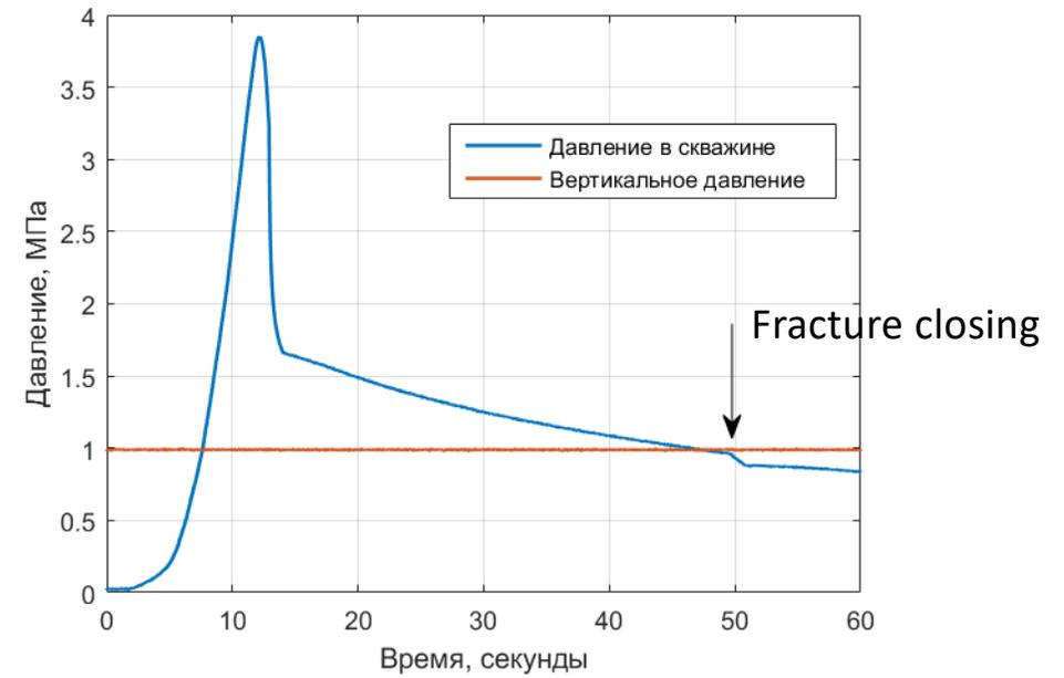
Vertical stress 1 MPa, horizontal stresses 0.2 MPa.
