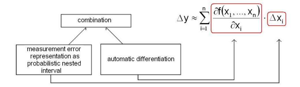
This combination can be easily programmed. Special library was written in C++ for linking with user projects and numerous tests were performed with it.
