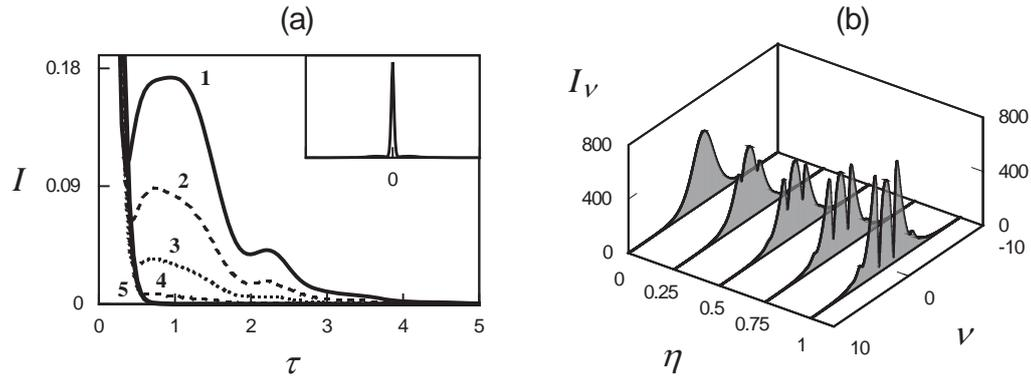
**Fig. 1.** (a) Soliton wing intensity  $I$  with varying lumped fractions of the saturable absorber: (1)  $\eta = 1$ , (2)  $\eta = 0.75$ , (3)  $\eta = 0.5$ , (4)  $\eta = 0.25$ , and (5)  $\eta = 0$ . (b) Soliton spectrum  $I_\nu$  with varying lumped fractions of the saturable absorber.
